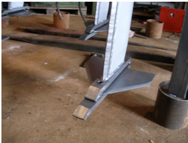
Figure 9. Working element of vibrating subsoiler VR-7
